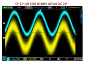
A small signal superimposed with a large DC results in a lower output noise and a higher SNR.
