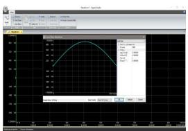
The arbitrary waveform editor has diversified generating method. The arbitrary waveform can be generated by insert the standard waveform or freely drawing.
