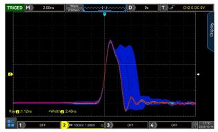
The new generation of wide dynamic high precision edge time adjustable pulse wave has a minimum pulse width of 2.4 ns. The pulse width can be fine adjusted and the minimum step is 100 ps. In addition, it can produce higher harmonic component, which has the feature of a dedicated pulse generator. The edge time can be set to a minimum of 1 ns independently.
