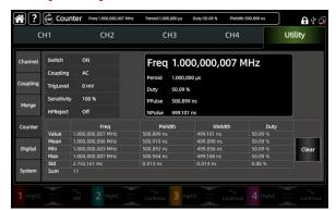
The high precision hardware frequency meter can measure the frequency range of 100 MHzto800 MHz.
