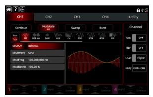
Modulating output (15 types): AM, FM, PM, DSB-AM, ASK, FSK, PSK, 3FSK, 4FSK, B PSK, Q PSK, OSK, SUM, QAM and PWM.
