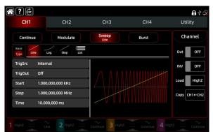
Four sweep frequency modes: "Linear", "Logarithm", "Step" and "List".
