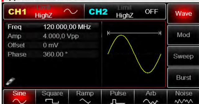
120MHz sine waveform output, Double Channel and Multiple Waveform Selection
