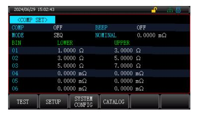
Built-in comparator BIN allows for setting comparison results for 6 BINs. The measured component can be divided into 7 BINs: BIN1, BIN2, BIN3, BIN4, BIN5, BIN6, and NG.
