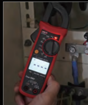
NCV multi-segment display and audio/visual alarm
