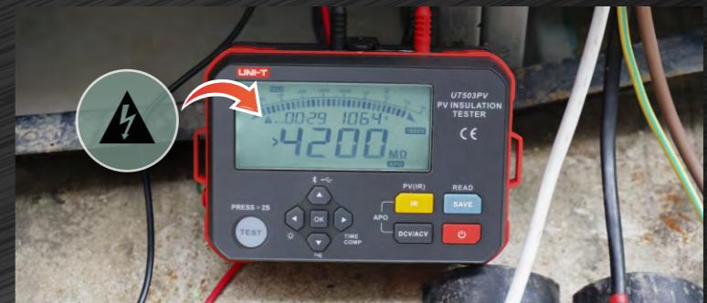
After measurement, the output voltage is turned off, the Tester discharges electricity automatically at a fast speed, and the LCD holds the present measurement information and data.
