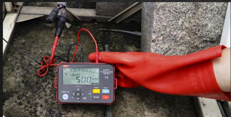
The maximum rated voltage between terminals is DC 1000V. Do not measure any energized equipment with a voltage of over DC 1000V, otherwise, it can cause electric shock or fault.
