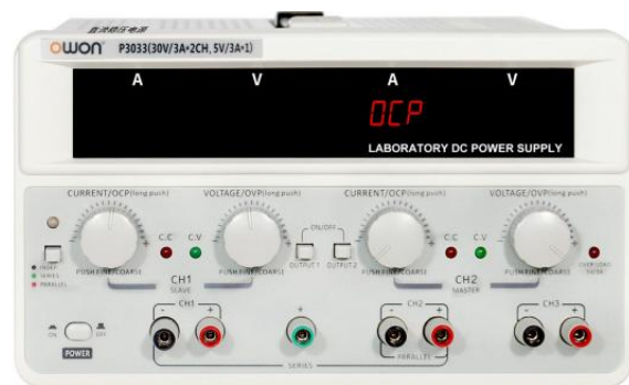
CH2 OCP Protection Alert
