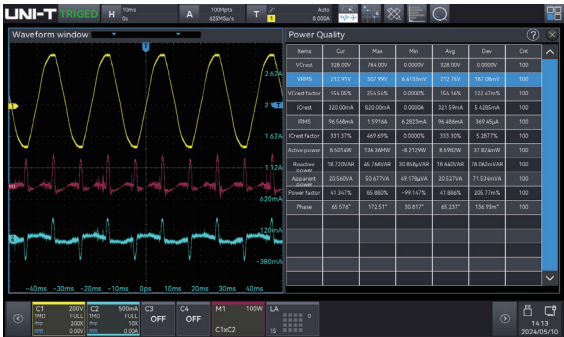
● Multiple power analysis functions: Power quality Harmonic analysis Switching loss Ripple wave analysis Loop analysis Safety operation area
