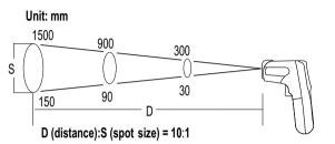
Make sure that the target is larger than the meter's visual spot size. The smaller the target, the closer you should be to it. The relationship between distance and spot size is 10:1
