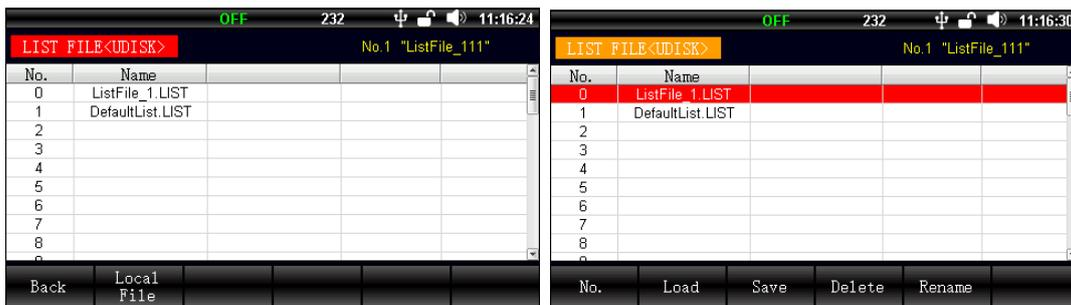
If press [Local File] shortcut key or plug out USB, the interface will switch to local page. File operation can be set via rotary knob or press arrow keys. The page only supports the operating of load, save, delete and rename. List File (Udisk) has parts of the operation similar to List File(Local).
